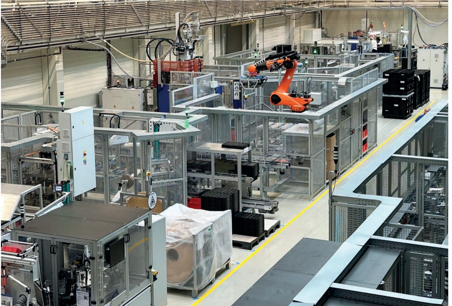
The automation equipment with a sophisticated transfer system encloses the injection molding machine.
