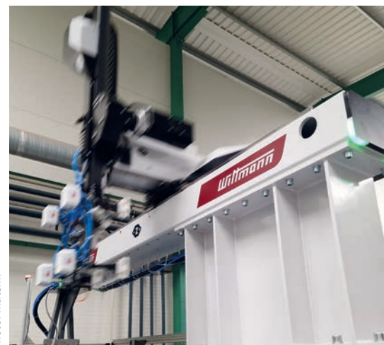
The Sonic high-speed robot contributes substantially to the high efficiency in the IML production of the rectangular 200-ml containers.
