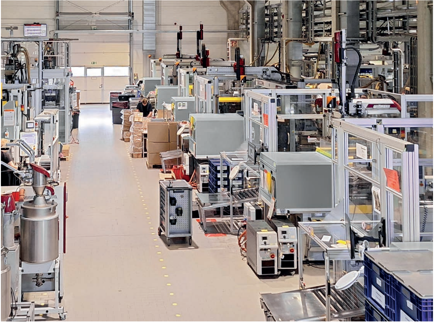
A total of 14 production cells are each equipped with a standardized automation cell.
