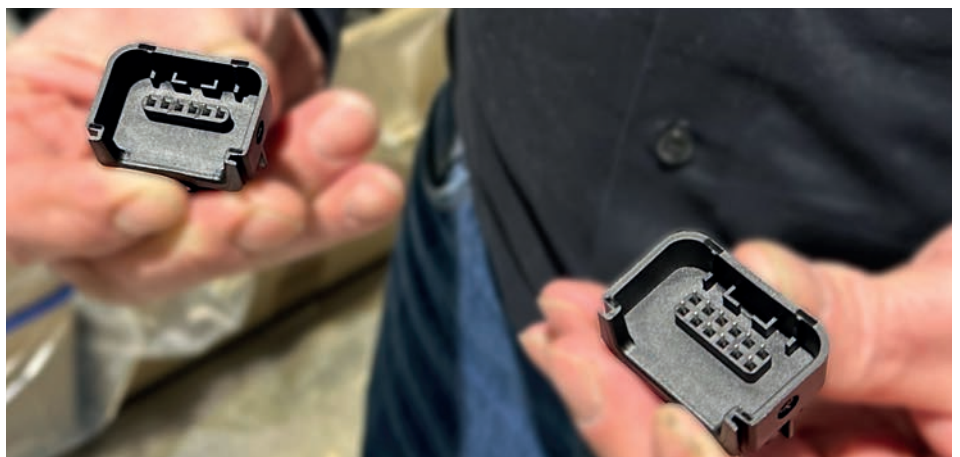
These plugs are used in automotive air suspension systems. Two different models are being produced.
