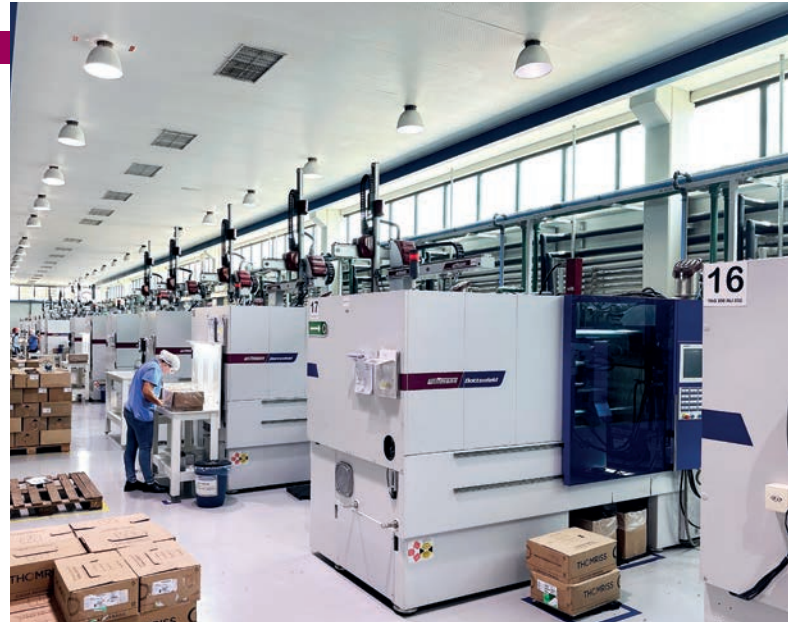
A total of 44 injection molding machines are up and running. The lion's share is taken up by servo-hydraulic SmartPower machines.
