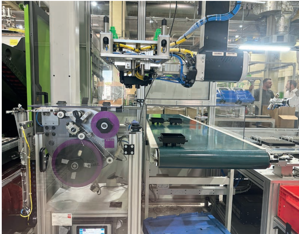
The camera for the fully automatic 100 per cent quality check is installed between the assembly station and the conveyor belt. Here, the W832 pro robot's rotary servo axes play out their strengths, for they are required to present in quick succession three different critical points.
