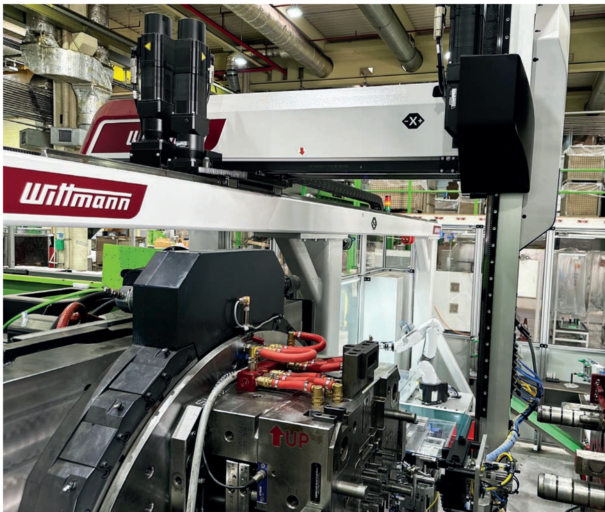
The W832 pro robot from WITTMANN is the link between injection molding and downstream processing steps.
