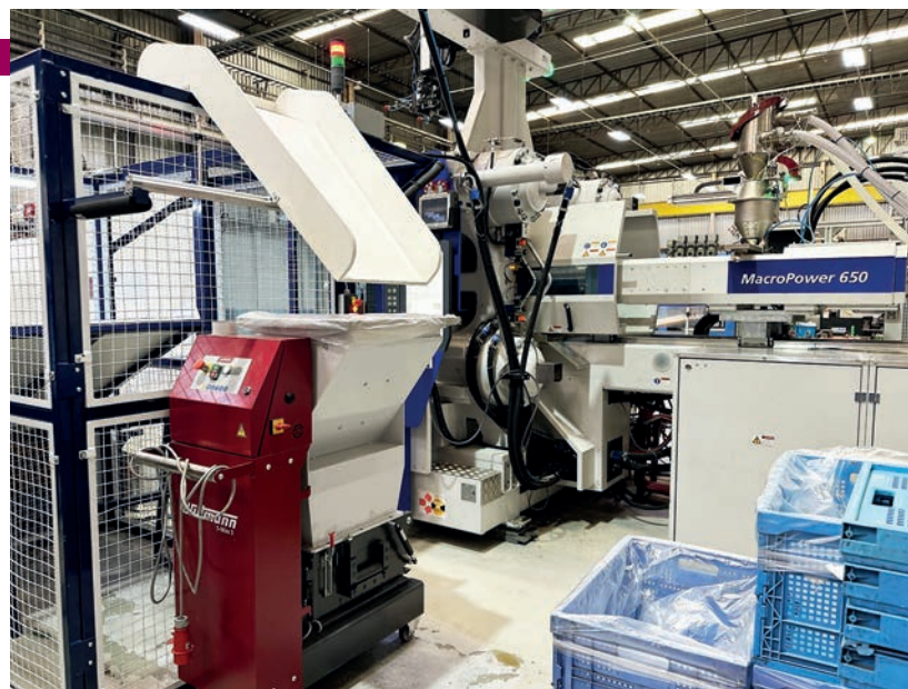
Sprue is partly reground directly beside the machine and subsequently re-processed.
