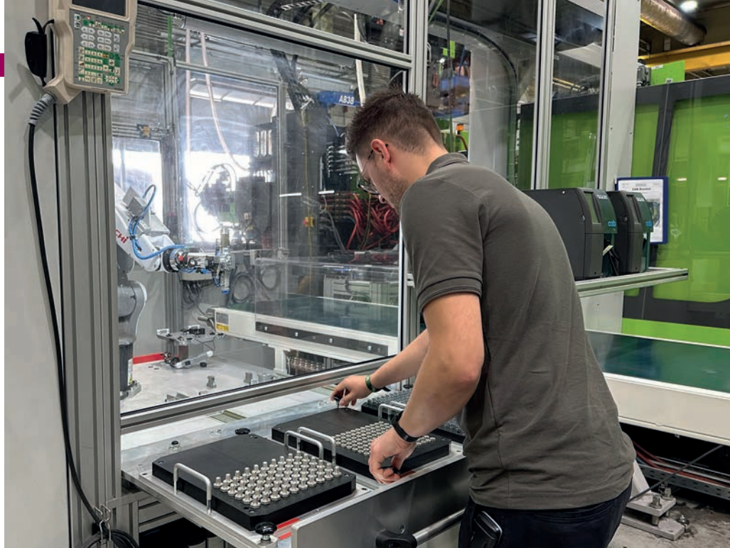
During the pre-series phase, the inserts are still being fed manually. But everything has been prepared for using vibrating bowls, hoppers and separators.
