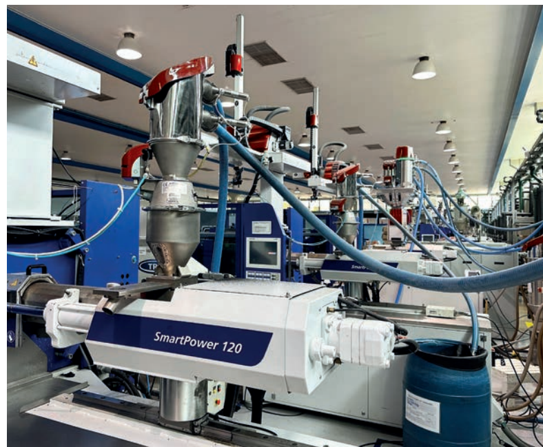
Everything from a single source: granulate feeding is handled exclusively by WITTMANN auxiliaries.
