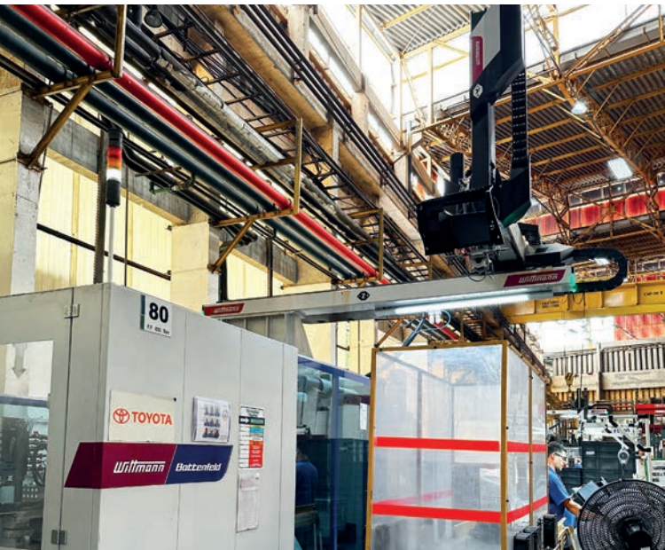
The glove compartments consist of two injection-molded components, a box and a lid, which are both produced on a MacroPower 650 injection molding machine.
