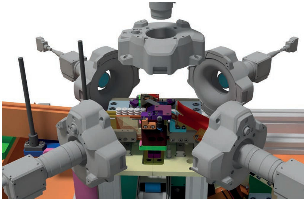
For fully automatic quality assurance, the automation engineers of WITTMANN BATTENFELD CZ integrated a total of five cameras into the fully automatic workplace for this application.
