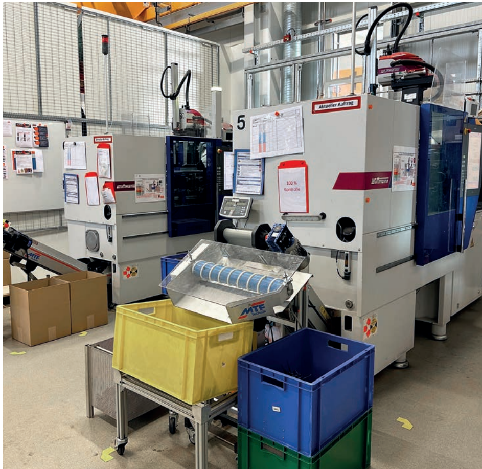
15 injection molding machines are installed at the plant. The newest machines are two SmartPower models from WITTMANN.
