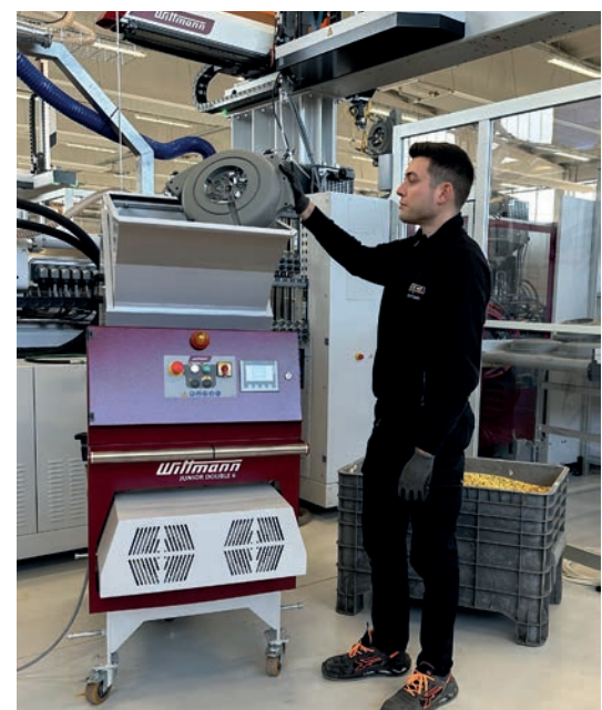
Sprue and reject parts are reground directly next to the machine.
