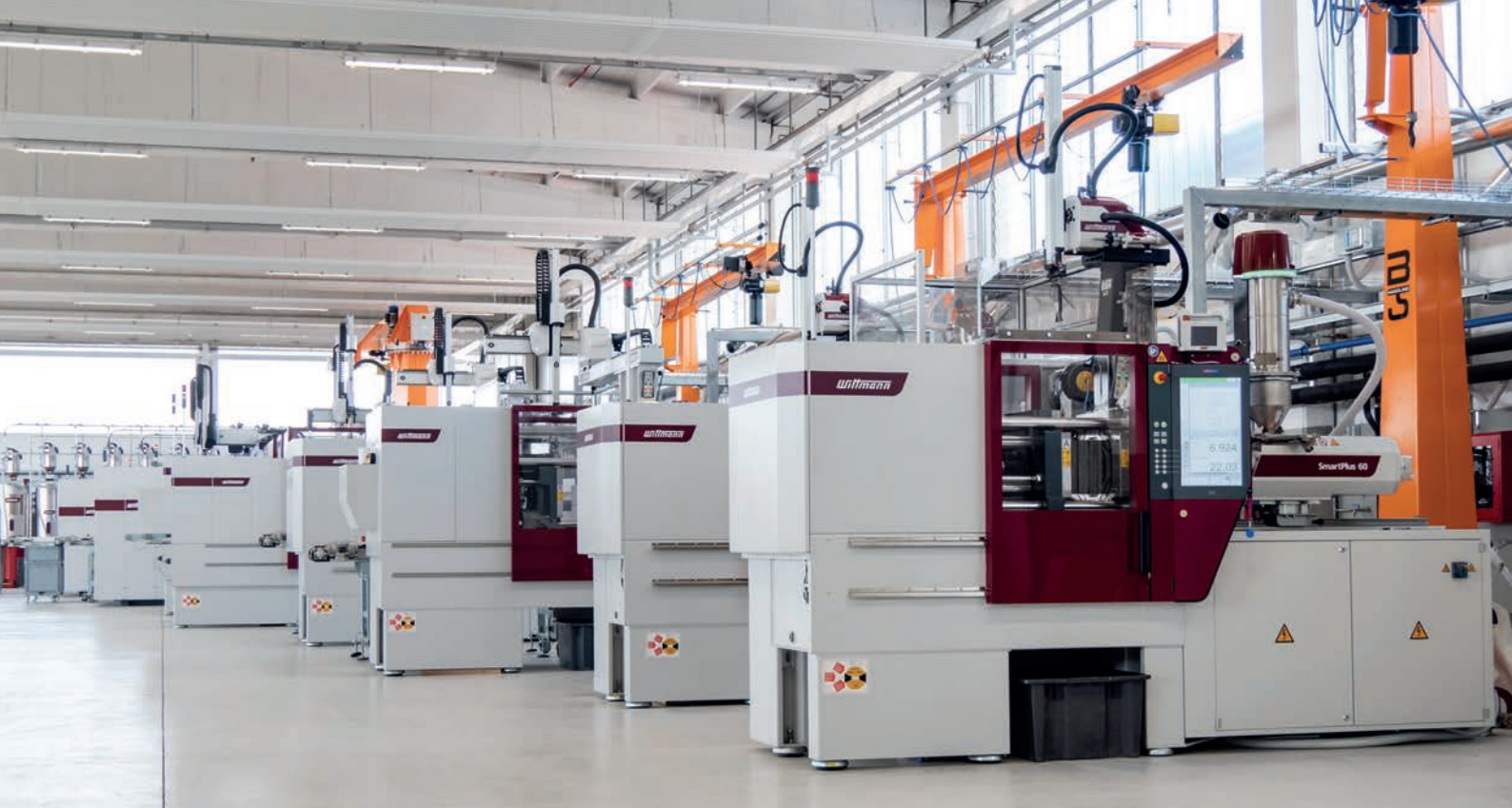
Top image: With eight automated and integrated injection molding machines from WITTMANN, ZECA has achieved great flexibility.
