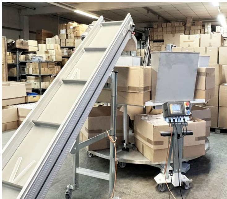
The two-level product carousel makes autonomous production for up to 18 hours possible.
