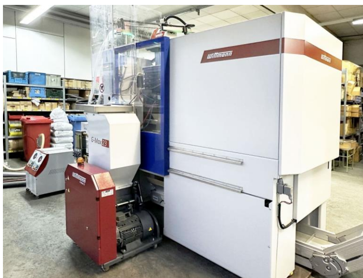
Spruce is granulated directly. For making the drugstore items, up to 10% regrind can be blended in with the virgin material.
