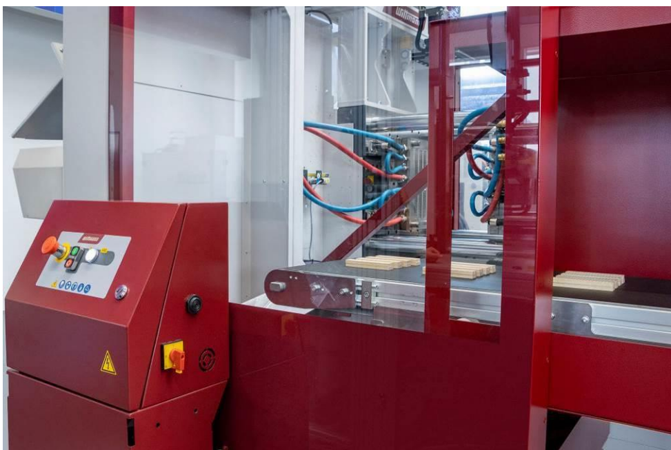
Fig. 4: WITTMANN S-Max granulator for spruce grinding
