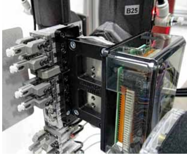
Left: WITTMANN W822 robot with micro-insert EOAT. Most insert molders with higher production runs are using horizontal injection presses with top-entry robots. Right: EOAT presenting parts to a single Cognex camera at lower right.
