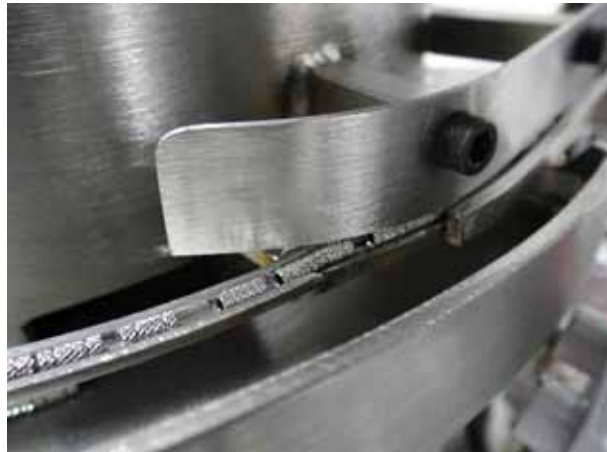
Left: Micro-grippers (shown holding inserts) are machined to very high tolerances and are often made of special materials based on application needs. Right: Micro-insert feeding will require more than a "garden-variety" bowl feeder.
