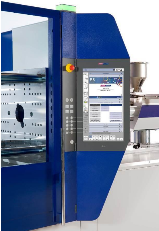
Fig. 1: The new UNILOG B8 control system – from the K 2016 onwards available for all PowerSeries machines
