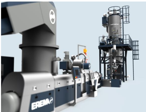
Picture 2: The combination of ReFresher and the proven TVEplus technology now offers odourless recyclates for the first time even in the case of severely contaminated packaging waste. Photocredit: EREMA
