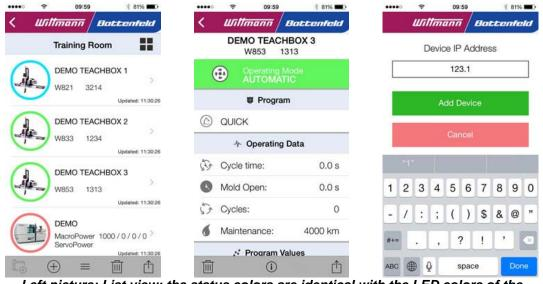
Left picture: List view; the status colors are identical with the LED colors of the WITTMANN W8 pro appliances; green stands for automatic operation, blue for non-automatic operation and red for safety criteria not complied with. Picture in the middle: Overview page on calling up an appliance in the automatic operation mode. Right picture: Addition of a new appliance; entry of an IP address.
